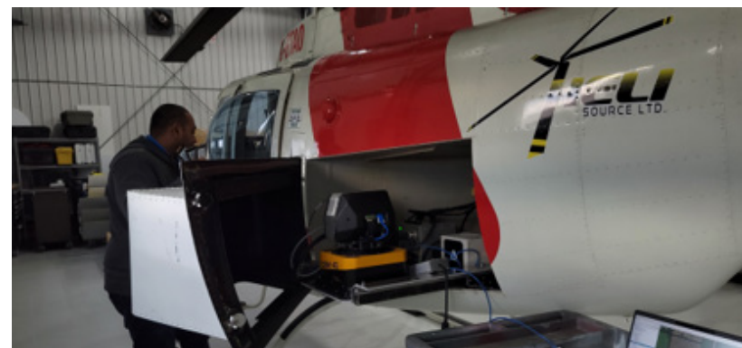
Figure 21: LSI's Infrared Hyperspectral Imaging System installed in a Bell 206 Helicopter
